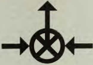
Figure 15-1.—This is the symbol used to indicate the differential in schematic drawings.
